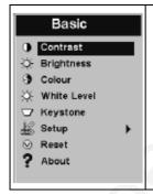
With the basic menu, you can set contrast, brightness, colour and keystoning or switch to the setup menu.
