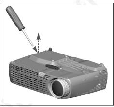
Open the lamp housing with a screw driver.
